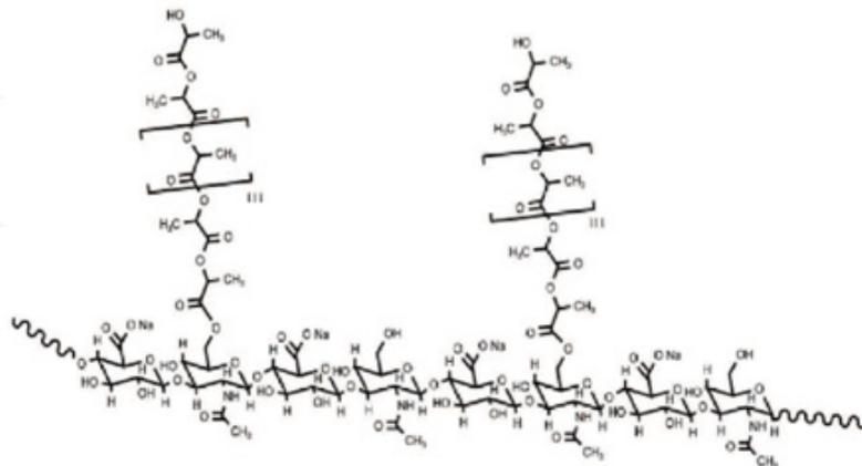
Fig. 1. Chemical structure of the HA-g-PLA copolymer
